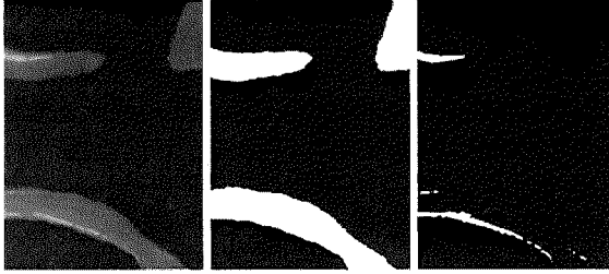
Figure 5.2: Image made from the top surface of the embedded bone specimen. left: original image, middle: segmented for bone, right: segmented for label.
