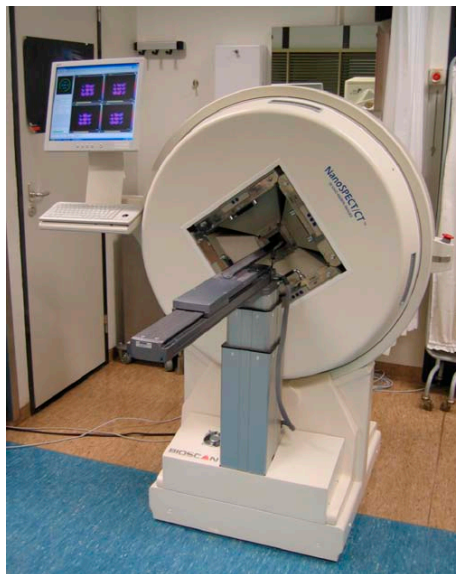
Fig. 1. The NanoSPECT (Bioscan Inc., Washington D.C., USA), a commercially available four-headed multiplexing multi-pinhole camera
