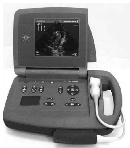
Figure 1 The OptiGo device, the hand carried cardiac ultrasound (HCU) device used in the study.
