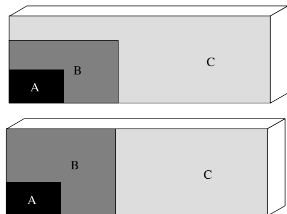
Fig. 3. Typical zone positioning for three classes in respectively square-in-time (upper part) and rectangular racks (lower part).
