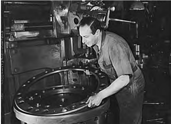
Figure 14 David Danzig, an Employee of the American Locomotive Company, Schenectady, New York, Applies the Fixture He Suggested and Designed for the Facing and Cutting Champer [sic; Clamper] on the Small Turret Ring for the M-4 Tank. Danzig was a plant award winner. Photographer: Howard R. Hollem. OWI, 1943, Library of Congress Prints and Photographs Division, call no. LC-USE6-D-008286 [P&P].
